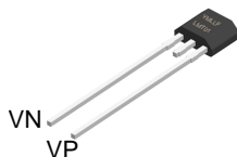
LPG Package 2-Pin TO-92 Top View
