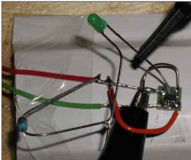
Figure 4. Picture of prototype blinking LED circuit.
