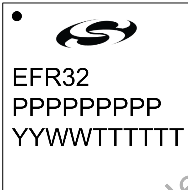
Figure 8.3. QFN32 Package Marking
